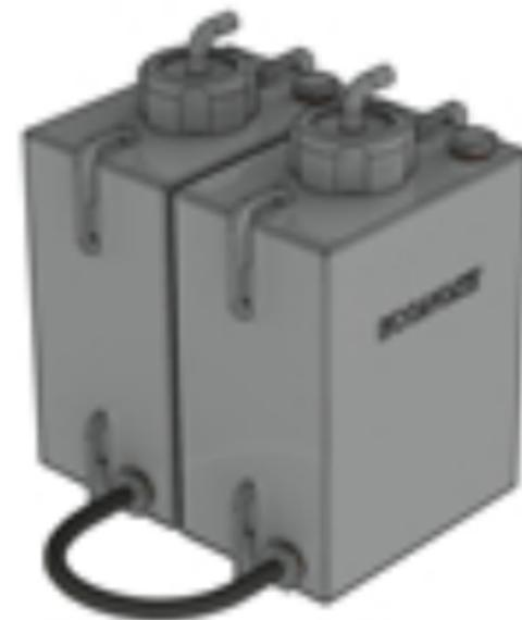
You have to respect the 2 following rules: you must connect the 2 bubblers L. The 2 bubblers must be continuously at the same height. See the drawings above. Make sure that the connection is water-proof. To do so, you need to complete screwing with a wrench; the gasket will have its full use.
